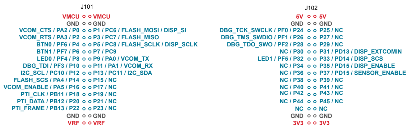
Figure 4.2. Radio Board Pin Mapping on Breakout Pads
